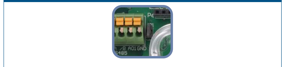
Fig. 5 Pull-up resistor jumper connected
